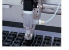
Epoxy sealing to smal relay
