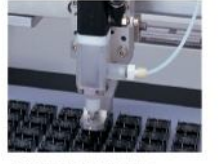
Epoxy sealing to small relay
