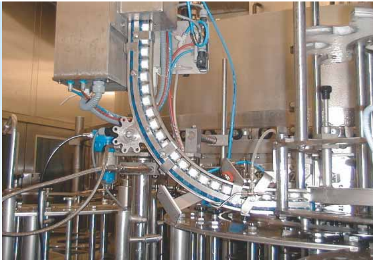
Disinfection of screw plugs in a drink filling plant
