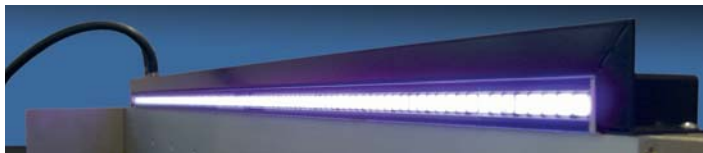
1.000 mm long LED array for printing applications
